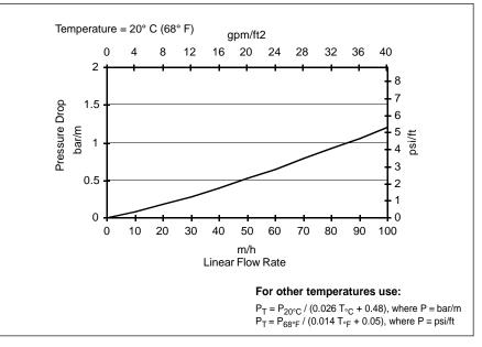
The data in Figure 2 shows the pressure drop per unit bed depth as a function of flow velocity. These figures are based on new resin which has been backwashed and settled and must be considered representative only. The total head loss of a unit in operation will also depend on the design, in addition to other factors such as level of fines and suspended solids. It is substantially affected by the contribution of the strainers surrounded by resin.
